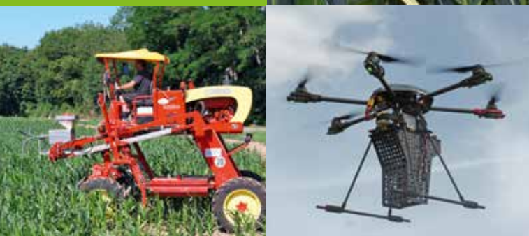
Pictures below: TRICHOSAFE®-capsule application with a stilt tractor and a drone
